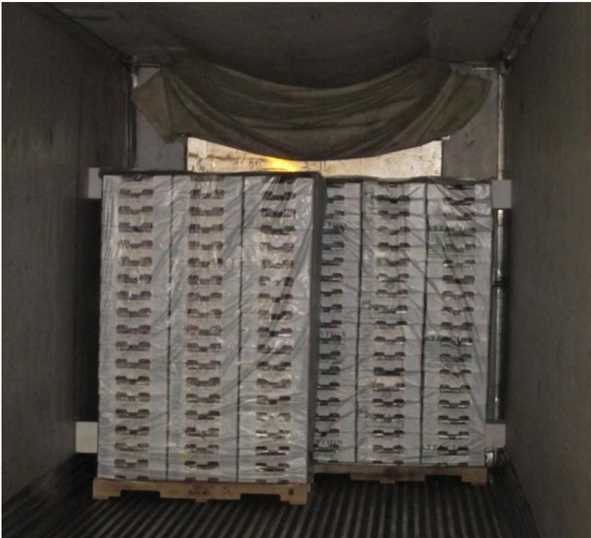
Fig. 4. Pallets of strawberries placed in pre-cooled trailer. The pallets have been overwrapped with PEAKfresh® strawberry pallet bags. Note that the bags are not sealed at the bottom and are open to airflow.
